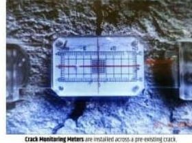
Crack Monitoring Meters are installed across a pre-existing crack. It measures if any expansion takes place in the crack.
