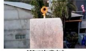
3 D Target for tilt check
