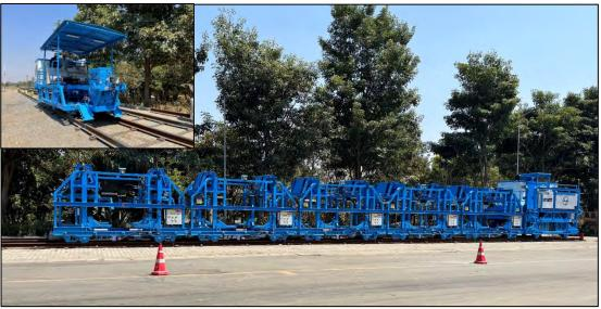
Track Works (package T2) -- Track Slab Laying Car and Rail Laying Car (In inset), Gujarat
